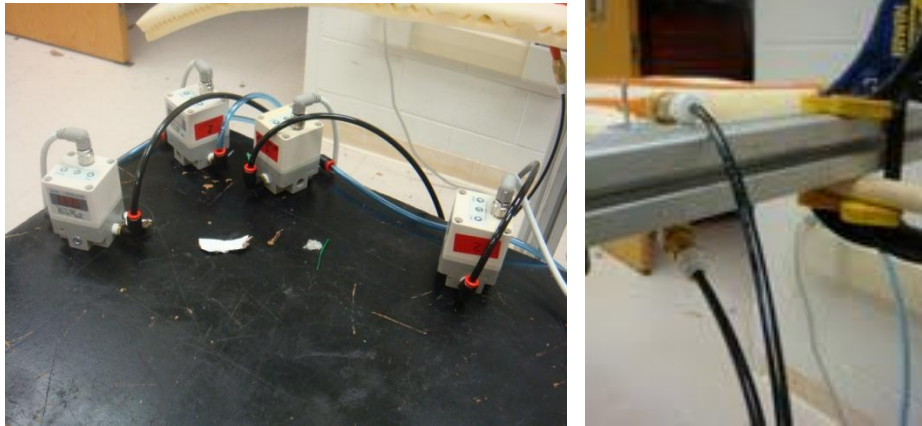
Pressure regulators and pneumatic lines from the air muscles
