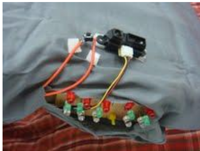
LEDs, IR sensor and push button at the side of table
